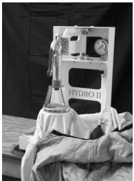
c. Engage the clamp by forcing the clamp handle in a downward direction until it latches in position.
