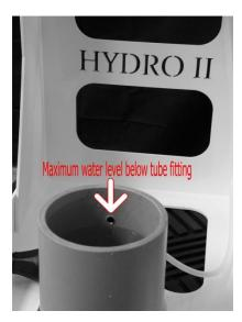
d. Fill the reservoir with clean water, filling to a point just below the tube fitting, located in the side of the reservoir.
