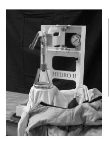
b. Swing the clamp arm back into position directly over the test area. Lower the clamp gently until the seal ring is resting on the garment. Make sure it is centered over the test area.
